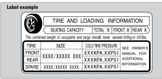
This figure includes the total weight of all occupants, cargo, and accessories, and the tongue load if you are towing a trailer. Below are the steps for determining the correct load limit:
