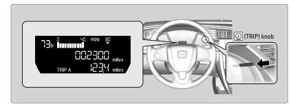
Press the TRIP knob to cycle through the displays, as shown below.
