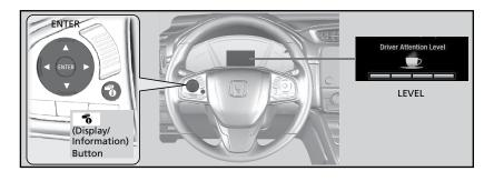
Driver attention is rated on a scale of 1 to 4, 4 being most attentive. If the system detects that attention is down to level 2, it will display a message.
