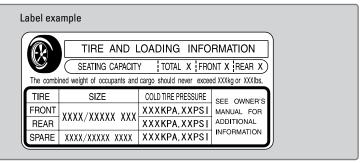
This figure includes the total weight of all occupants, cargo, and accessories, and the tongue load if you are towing a trailer. Below are the steps for determining the correct load limit:
