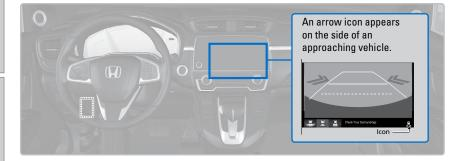
The system does not provide alerts for a vehicle that is moving away from your vehicle, and it may not detect pedestrians, bicycles, or stationary objects.
