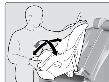
7. Make sure any unused seat belt that a child can reach is buckled, the lockable retractor is activated, and the belt is fully retracted and locked.
