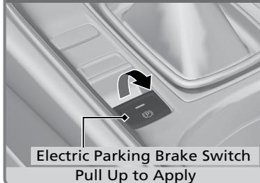
Automatic transmission/Continuously variable transmission models
