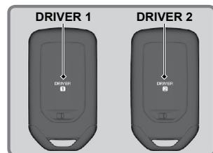
When you unlock and open the driver's door with a remote transmitter, the seat adjusts automatically to one of the two preset positions.
