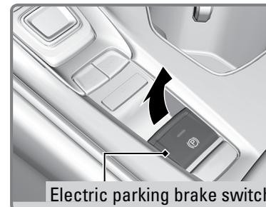
**To release:** The power mode must be in ON in order to release the electric parking brake.
