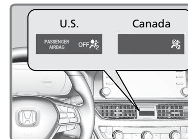
If the front passenger's seat is empty, the indicator will come on and, in the event of a crash, the front passenger's airbag will not deploy. The front passenger's knee airbag will not deploy either.
