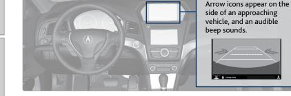
The system does not detect or provide alerts for a vehicle that is moving away from your vehicle, and it may not detect pedestrians, bicycles, or stationary objects.
