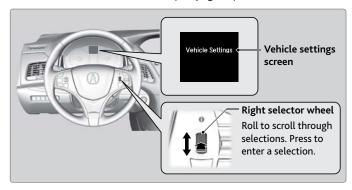
An example of how to change the Trip A reset timing setting is below. Use the right selector wheel to make and enter selections.
