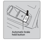
To turn off brake hold: Press the brake pedal and press the BRAKE HOLD button
