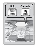
If the indicator comes on with no occupant or objects in the front passenger's seat, something may be interfering with the weight sensors, such as:
