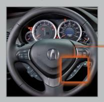
Press and hold either INFO button (▲/▼) to enter customization mode, then press SEL/RESET to enter the menu.
