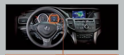
When you start the engine, the MID shows the last active lower display from the previous drive cycle.
