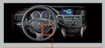
To toggle between the different displays, press either Info button (▲/▼) for the main displays and press the SEL/RESET button for the lower displays.
