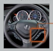
Press and hold either INFO button (▲/▼) to enter customization mode, then press SEL/RESET to activate the menu.
