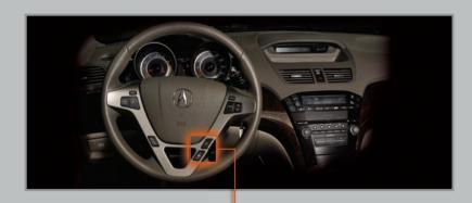
While on the Trip Computer display, press SEL/RESET to access trip information and to toggle through the various screens. Press either INFO (▲/▼) button to return to the Trip Computer main display.
