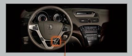
To toggle between the different displays, press either Info button (▲/▼) for the main displays and press SEL/RESET for the lower displays.
