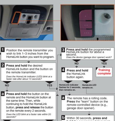
hold the programmed HomeLink button for 2 seconds. 5 **Press** the programmed HomeLink button again; the remote-controlled device should operate.
