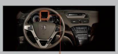
When you start the engine, the MID shows the last active display from the previous drive cycle.
