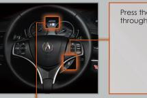
Press the Distance button to shuffle through four ranges.
