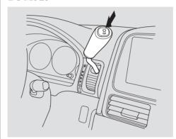
Press the D3 switch on the edge of the shift lever to turn this mode on or off; the D3 mode indicator comes on whenever the D3 mode is selected.
