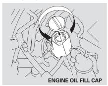
Unscrew and remove the engine oil fill cap on the valve cover. Pour in the oil slowly and carefully so you do not spill any. Clean up any spills immediately. Spilled oil could damage components in the engine compartment. Reinstall the engine oil fill cap, and tighten it securely. Wait a few minutes, and recheck the oil level on the engine oil dipstick. Do not fill above the upper mark; you could damage the engine.
