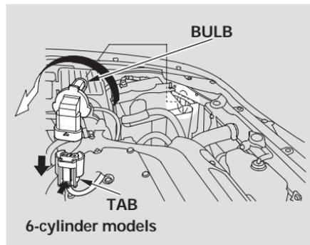
5. Push the electrical connector onto the bulb.
