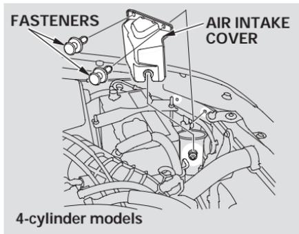
1. Open the hood. To change a bulb on the passenger's side, undo the two fasteners and remove the air intake cover.
