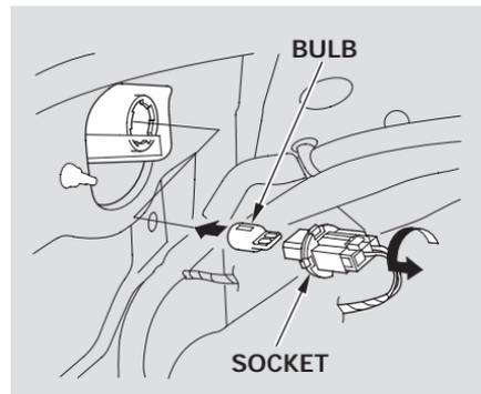
3. Remove the socket by turning it one-quarter turn counterclockwise, and pull the bulb straight out of its socket.
