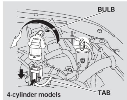
3. Remove the bulb by turning it approximately one-quarter turn counterclockwise.
