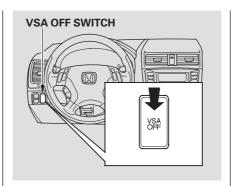
This switch is under the left vent. Press it to turn the VSA system on and off.
