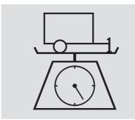
Total Trailer Weight: The maximum allowable weight of the trailer and everything in or on it must not exceed 1,000 lbs (450 kg). Towing a load that is too heavy can seriously affect your vehicle's handling and performance. It can also damage the engine and drivetrain
