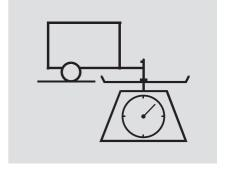
Tongue Load: The weight that the tongue of a fully-loaded trailer puts on the hitch should be approximately 10 percent of the trailer weight. Too much tongue load reduces front-tire traction and steering control. Too little tongue load can make the trailer unstable and cause it to sway.
