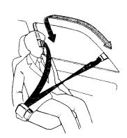
2. Turn the ignition ON. The shoulder belt buckle will move to its rear locked position. The length of the shoulder belt will adjust automatically to your body and seating position.
