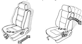
The angle of the seat-back can be changed by pulling up on the lever at the outside edge of the seat and leaning forward or back. Release the lever and let the seat lock into place when it reaches the desired angle.
