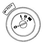
0-LOCK position: The key can be removed or inserted in this position. To remove the key, push it in at position I, then turn it to 0 and pull it out. When the key is removed, the steering column will lock.
