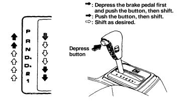
If you cannot shift out of Park with the brake pedal depressed and the ignition switch in the II position:
