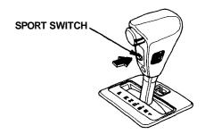
NOTE: Although the S indicator light in the instrument panel will come on in any gear range when the Sport switch is pushed, this mode is selectable only in the D<sub>3</sub> and D<sub>4</sub> range.
