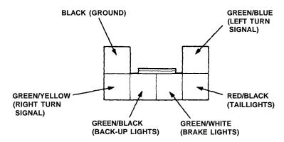
To connect your car's taillights to a trailer, an electrical converter must be installed in the car. Your car has separate bulbs for brake (red) and turn signal lights (amber), while most trailers use the same bulb for brake and turn signal lights. A converter, available at most trailer supply stores, should be installed according to the instructions supplied by the converter manufacturer.
