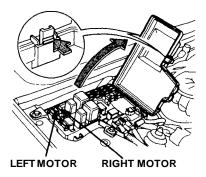
3. If the fuse has blown, replacing it with a new fuse of the same amperage should allow the shoulder belt buckle motor to work. However, if the fuse hasn't blown, or if a new fuse did not solve the problem, remove the fuse and operate the motor manually.
