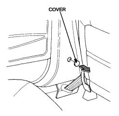
5. Set the wrench extension into the wrench grip (both provided in the tool bag) then insert the wrench into the socket and turn it counterclockwise until the shoulder belt buckle reaches its rear locked position.
