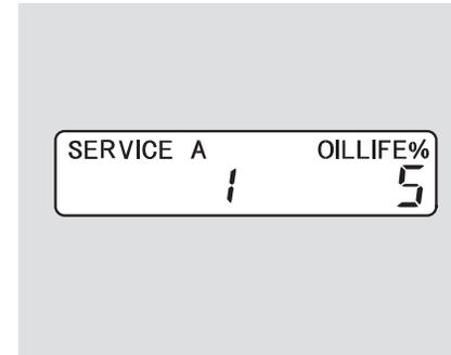
When the remaining engine oil life is 5 to 1 percent, you will see a “SERVICE” message along with the same maintenance item code(s), every time you turn the ignition switch to the ON (II) position.
