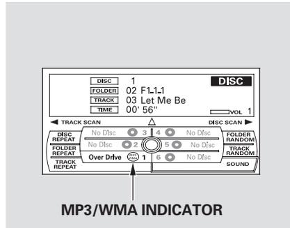
Using the interface selector, you can see the list of all the files and folders within a disc. While playing a MP3/WMA disc, press the AUDIO button. The currently playing folder and file information comes on the screen.
