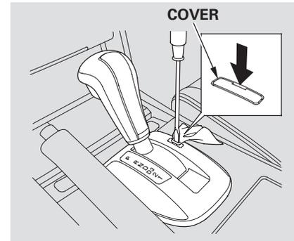
3. Put a cloth on the edge of the shift lock release slot cover. Use a small flat-tipped screwdriver or metal fingernail file to carefully pry up the edge of the cover and remove it from the slot.
