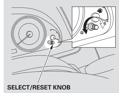
The select/reset knob on the instrument panel controls the brightness of the instrument panel lights. Turn the knob to adjust the brightness with the ignition switch in the ON (II) position and the parking lights on.
