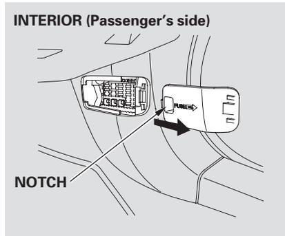
The passenger's side interior fuse box is on the lower right side panel. To remove the fuse box lid, put your finger in the notch on the lid, and pull it upward slightly, then pull it toward you and take it out of its hinges.
