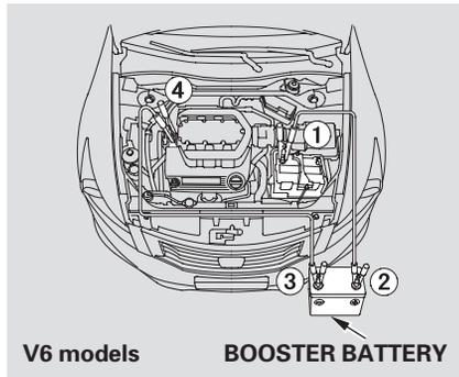
3. Connect one jumper cable to the positive (+) terminal on your battery. Connect the other end to the positive (+) terminal on the booster battery.
