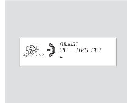
4. Turn the selector knob to select the item which you want to adjust. Turning the knob will change the selected item between the clock display setting, hours, minutes, and SET. The selected item is indicated with  $\triangle$  in the display.
