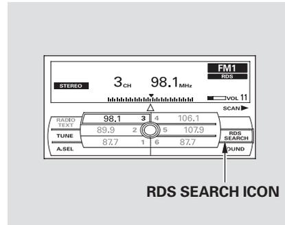
On the FM band selected, you can select the program type provided by the RDS. Press the AUDIO button to display the radio information on the screen. Push down the selector on the interface dial, then turn the knob to select RDS SEARCH icon. Press ENTER to set your selection. The principal RDS categories are shown as follows;
