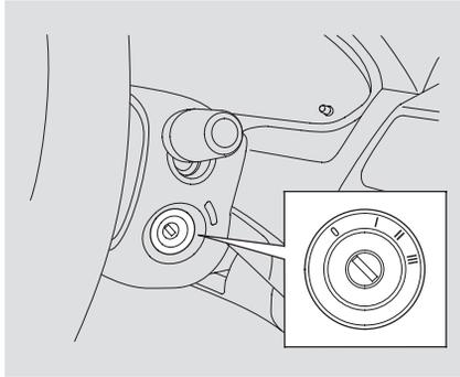
The ignition switch has four positions: **LOCK (0)**, **ACCESSORY (I)**, **ON (II)**, **START (III)**
