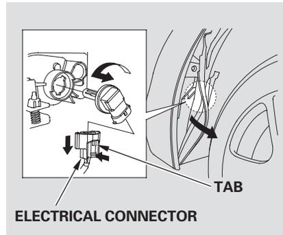
6. Remove the electrical connector from the bulb by pushing on the tab and pulling the connector down.
