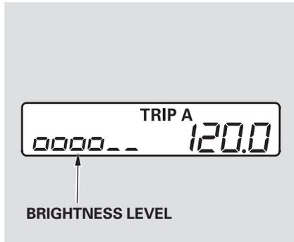
The level of brightness is shown on the information display while you adjust it. It goes out about 5 seconds after you finish adjusting.
