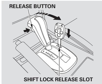
5. Push down on the key while you press the release button on the front of the shift lever and move the shift lever out of Park to neutral.
