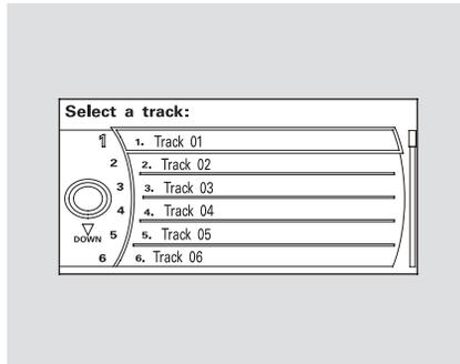
You can also choose a track directly from a track list. Press ENTER on the interface selector, and the track list screen will be shown. If there are no track names, track numbers are displayed. You will see the current track is highlighted. Turn the interface knob to select the desired track, then press ENTER on the interface selector.
