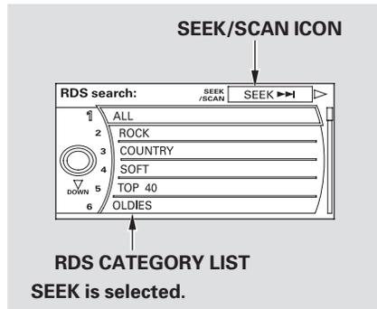
To activate RDS program search with the interface dial, push the AUDIO button to display the FM radio information on the screen. Push the selector down, and turn the knob to select RDS SEARCH icon. Press ENTER on the selector. The screen shows you the RDS category list.
