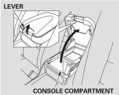
To open the console compartment, pull up on the lever and lift the armrest.
