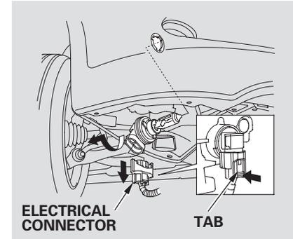
2. Remove the electrical connector from the bulb by pushing on the tab to unlock it, then slide the connector off the bulb.
