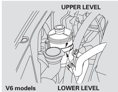
Pour the fluid slowly and carefully so you do not spill any. Clean up any spills immediately; it could damage components in the engine compartment.
