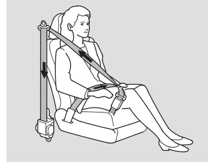
For added protection, the front seat belts are equipped with automatic seat belt tensioners. When activated, the tensioners immediately tighten the belts to help hold the driver and a front passenger in position.
