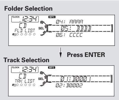
In MP3 or WMA mode, you can also select a folder or track/file from the list by using the selector knob. Push the selector knob (ENTER) to switch the display to the list displayed with three segments, then turn the knob to select a folder. Press the selector knob (ENTER) to change the display to the track/file list, then turn the same knob to select a track/file. Press the selector knob (ENTER) to set your selection.
