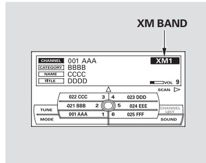
**Preset** – You can store up to 12 preset channels using the six preset buttons. Each button stores one channel from the XM1 band and one channel from the XM2 band.
