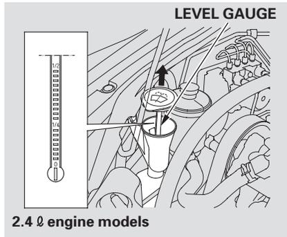
Check the level in the windshield washer reservoir at least monthly during normal use.
