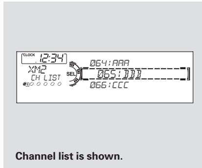
You can also select a channel or category from the list by using the selector knob. Push the selector knob (ENTER) to switch the display to the list displayed with three segments, then turn the knob to select a channel or category. Press the selector knob (ENTER) to set your selection.
