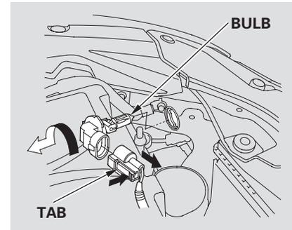
2. Remove the electrical connector from the bulb by pushing on the tab to unlock it, then slide the connector off the bulb.
