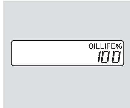
4. Press the select/reset knob for another 5 seconds. The maintenance item code(s) will disappear, and the engine oil life will reset to "100."
