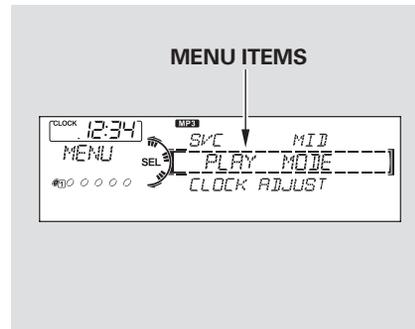
You can select any type of repeat, random and scan modes by using the MENU button and the selector knob. Push the MENU button to display the menu items, then turn the selector knob to select “PLAY MODE.” Press the selector knob (ENTER) to set the selection.
