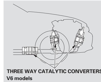
**THREE WAY CATALYTIC CONVERTERS**
