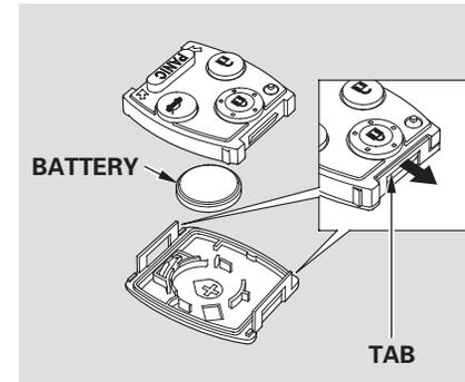
3. Inside the transmitter, separate the inner cover from the keypad by releasing the two tabs on the cover.
