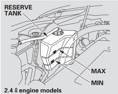
Look at the coolant level in the radiator reserve tank. Make sure it is between the MAX and MIN lines. If it is below the MIN line, see **Adding Engine Coolant** on page 320 for information on adding the proper coolant.
