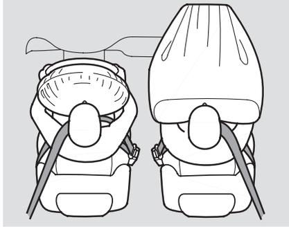
Your vehicle has a supplemental restraint system (SRS) with front airbags to help protect the heads and chests of the driver and a front seat passenger during a moderate to severe frontal collision (see page 23 for more information on how your front airbags work).
