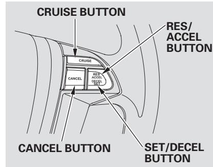
1. Push in the CRUISE button on the steering wheel. The CRUISE MAIN indicator on the instrument panel comes on.
