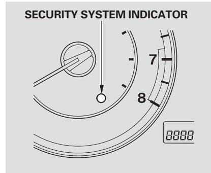
Once the security system is set, opening any door (without using the key or the remote transmitter), the hood, or the trunk will cause the system to alarm. It also alarms if the audio unit is removed from the dashboard or the wiring is cut.
