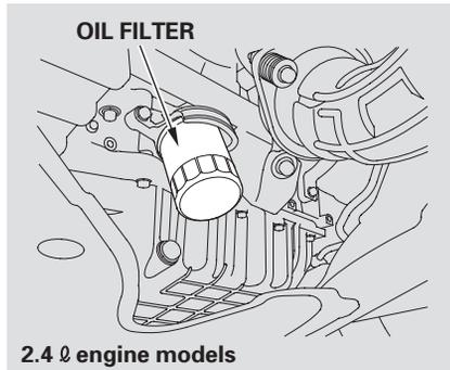
4. Install a new oil filter according to the instructions that come with it. Make sure to clean off any dirt and dust on the connecting surface of a new oil filter.
