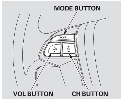
Three controls for the audio system are mounted in the steering wheel hub. These let you control basic functions without removing your hand from the wheel.
