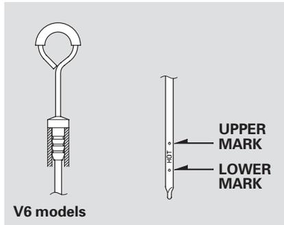
4. Remove the dipstick and check the fluid level. It should be between the upper and lower marks.
