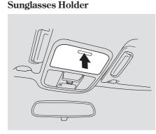
To open the sunglasses holder, push on the front edge. It will unlatch and swing down. To close it, push it until it latches. Make sure the holder is closed while you are driving.
