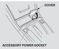
Your car has two accessory power sockets, one is located in the front of the center console, and the other is in the center console compartment. To use an accessory power socket, the ignition switch must be in ACCESSORY (I) or ON (II).
