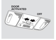
*On EX and EX-V6 models* The spotlights have a two-position switch. In the DOOR position, the lights come on when you open either door. In the OFF position, the lights do not come on. The spotlights (with the switch in the DOOR position) also come on when you unlock the door with the remote transmitter, and when you remove the key from the ignition switch. (See Ceiling Light on page 117.)
