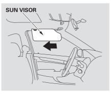
*On cars with side curtain airbags* In this position, the sun visor can be adjusted by moving it on its slider. Do not use the sun visor over the rear view mirror. Make sure you put the sun visor back in place when you are getting into or out of the car.
