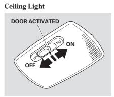
The ceiling light has a three-position switch. In the OFF position, the light does not come on. In the center position, the ceiling light comes on when you open either door. After both doors are closed tightly, the light dims slightly, then fades out in about 30 seconds. In the ON position, the ceiling light stays on continuously.
