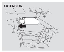
*On cars without side curtain airbags* In this position, the sun visor can be extended by sliding out the extension. Do not use the sun visor extension over the rear view mirror.
