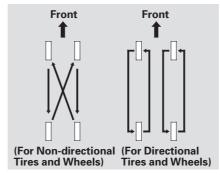
To help increase tire life and distribute wear more evenly, you should have the tires rotated every 10.000 miles (16.000 km) on 4-cylinder models and 7.500 miles (12,000 km) on 6-cylinder models. Move the tires to the positions shown in the chart each time they are rotated.
