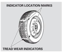
Your car's tires have wear indicators molded into the tread. When the tread wears down to that point, you will see a 1/2 inch (12.7 mm) wide band running across the tread. This shows there is less than 1/16 inch (1.6 mm) of tread left on the tire. A tire that is this worn gives very little traction on wet roads. You should replace the tire if you can see the tread wear indicator in three or more places around the tire.
