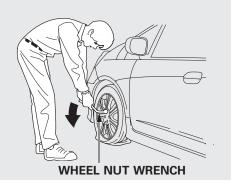
9. Loosen each wheel nut 1/2 turn with the wheel nut wrench.
