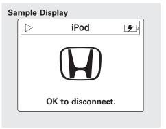
When the iPod is connected and the iPod mode is selected on the audio display, the iPod indicator is shown on the screen. After loading, you will see Honda mark\* on the iPod. That means you can only operate your iPod using the vehicle's audio unit.
