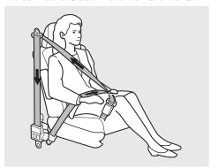
For added protection, the front seat belts are equipped with automatic seat belt tensioners. When activated, the tensioners immediately tighten the belts to help hold the driver and a front passenger in position. The tensioners are designed to activate in any collision severe enough to cause the front airbags to deploy.
