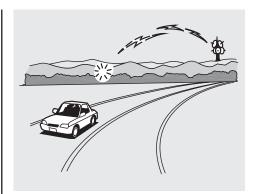
Driving very near the transmitter of a station that is broadcasting on a frequency close to the frequency of the station you are listening to can also affect your radio's reception. You may temporarily hear both stations, or hear only the station you are close to.
