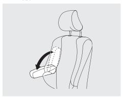
On Sport model and Canadian LX model The driver's seat has an armrest on the side of the seat-back. To use, pivot it down.
