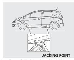
10. Place the jack under the jacking point nearest the tire you need to change. It is pointed to by a △ mark molded into the underside of the body (Sport model). Turn the end bracket clockwise until the top of the jack contacts the jacking point. Make sure the jacking point tab is resting in the jack notch.
