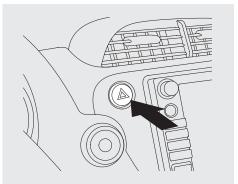
Push the button to turn on the hazard warning lights (four-way flashers). This causes all four outside turn signals and both turn indicators in the instrument panel to flash. Use the hazard warning lights if you need to park in a dangerous area near heavy traffic, or if your vehicle is disabled.
