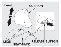
Adjusting the Head Restraint
