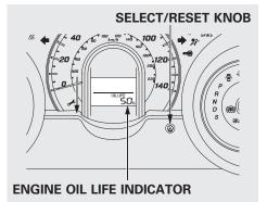
To see the current engine oil life, turn the ignition switch to the ON (II) position, then press and release the select/reset knob repeatedly until the engine oil life indicator appears (see page 68).
