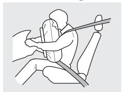
If you ever have a moderate to severe frontal collision, sensors will detect the vehicle's rapid deceleration.
