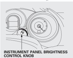
You can change the instrument panel brightness only when the ignition switch is in the ON (II) position and the light switch is on.
