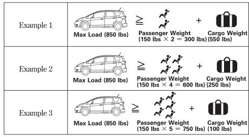
In addition, the total weight of the vehicle, all occupants, accessories, cargo, and trailer tongue load must not exceed the Gross Vehicle Weight Rating (GVWR) or the Gross Axle Weight Rating (GAWR). Both are on a label on the driver's doorjamb.
