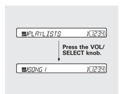
You can also select a file from any list on the iPod menu: playlists, artists, albums and songs, by using the VOL/SELECT knob. Push the VOL/SELECT knob to switch the display to an iPod menu, then turn the VOL/SELECT knob to select a desired list. Press the VOL/SELECT knob to set your selection.
