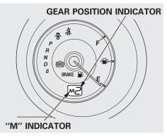
When you move the shift lever from "D" to the "S" position and pull either paddle shifter, the gear position indicator displays "M" along with the selected gear number.
