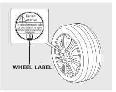
15. Remove the wheel label from the repair kit, wipe any dirt off the wheel with a clean cloth, and attach the label to the center of the wheel.
