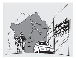
Radio reception can be affected by atmospheric conditions such as thunderstorms, high humidity, and even sunspots. You may be able to receive a distant radio station one day and not receive it the next day because of a change in conditions. Electrical interference from passing vehicles and stationary sources can cause temporary reception problems.
