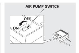
10. Turn the air pump on to inflate the tire. Do not run the air pump for more than 15 minutes or it may overheat. The air pressure gauge will show about 40 to 60 psi (275 to 415 kPa) for the first few minutes while the sealant is pumped into the tire, and then the pressure will go down to about 10 to 20 psi (70 to 140 kPa).
