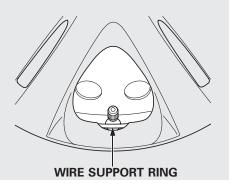
3. Make sure the wire support ring is on the outer side of the tire valve as shown.
