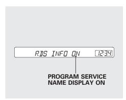
To switch the function between on and off, press and release the TITLE button. With the system on, you will see the "RDS INFO ON" message on the display. If the station you are listening to is an RDS station, the displayed frequency switches to the station name.
