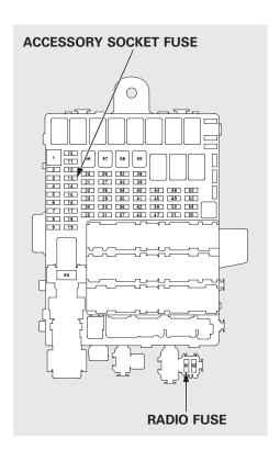
Only remove the fuses after you have performed the transmission shifting procedure, and the key is in the ACCESSORY (I) position. Store the fuses in an obvious location (center pocket, etc) as a reminder to reinstall the fuses before driving the vehicle.
