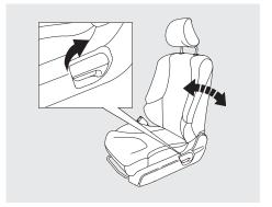
To change the seat-back angle, pull up the lever on the outside of the seat bottom.
