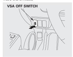
This switch is under the driver's side beverage holder. To turn the VSA system on and off, press and hold it until you hear a beep.
