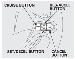
1. Press the CRUISE button on the steering wheel. The CRUISE MAIN indicator on the instrument panel comes on.
