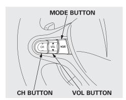
On vehicles with navigation system Three controls for the audio system are mounted in the steering wheel hub. These let you control basic functions without removing your hand from the wheel. The VOL button adjusts the volume up (♠) or down (▼). Press the top or bottom of the button and hold it until the desired volume is reached, then release it.
