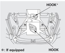
The two or four hooks on the floor can be used to install a net for securing items.
