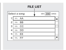
After the system searches for a song, a file list is displayed. To scroll through the list, touch the ▲ or ▼ icon on the side of the screen. Select the desired file by touching the appropriate icon, or moving the joystick and pressing the ENT.
