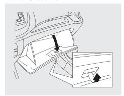
Open the lower glove box by pulling the bottom of the handle. Close it with a firm push.
