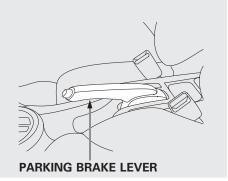
To apply the parking brake, pull the lever up fully. To release it, pull up slightly, push the button, and lower the lever. The parking brake indicator on the instrument panel should go out when the parking brake is fully released (see page 60).
