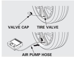
20. Stop safely and check the pressure in the tire. Remove the tire valve cap, screw the air pump hose onto the tire valve, and check the air gauge. (You do not need to attach the power cord or turn the air pump switch on.)
