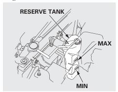
Look at the coolant level in the radiator reserve tank. Make sure it is between the MAX and MIN lines. If it is below the MIN line, see **Adding Engine Coolant** on page 256 for information on adding the proper coolant.
