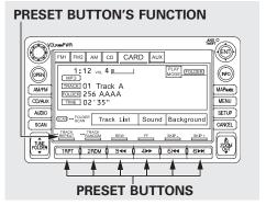
You can use the preset buttons while a card is playing to select or change files. Each preset button's function is shown on the bottom of the screen. Icons on the screen can also be selected with the joystick. Move the joystick left or right and up or down until the icon is highlighted, then press the ENT on the top of the joystick to select the icon.
