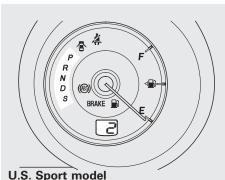
These indicators on the instrument panel show which position the shift lever is in.
