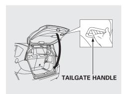
To close the tailgate, hold the tailgate handle, lower the tailgate, then press down on the back edge.
