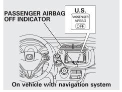
This indicator alerts you that the passenger's front airbag has been shut off because weight sensors detect about 65 lbs (29 kg) or less (the weight of an infant or small child) on the front passenger's seat. It does *not mean* there is a problem with the airbag.
