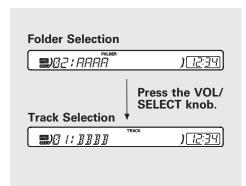
You can also select a folder or file by using the VOL/SELECT knob. Push the VOL/SELECT knob to switch the display to the folder or file list, then turn the VOL/SELECT knob to select a folder or file. Press the VOL/SELECT knob to set your selection.
