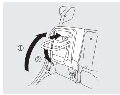
Pull up the rear seat cushion, and fold the seat leg down. Push the seat cushion firmly against the seat-back to lock it.
