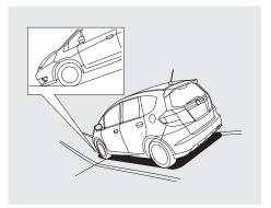
• Curbs and steep inclines could damage the front and rear bumpers. Low curbs that do not affect the average vehicle may be high enough to hit the bumper on your vehicle. The front or rear bumper may scrape when trying to drive onto an incline, such as a steep driveway or trailer ramps.
