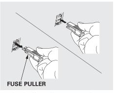
4. Check all smaller fuses in the interior fuse box by pulling out each one with the fuse puller provided in the interior fuse box.
