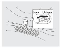
Push the release lever to the right as shown.
