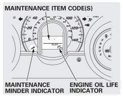
If the remaining engine oil life is 15 to 6 percent, you will see the engine oil life indicator every time you turn the ignition switch to the ON (II) position. The maintenance minder indicator will also come on, and the maintenance item code(s) for other scheduled maintenance items needing service will be displayed above the "OIL LIFE" message.
