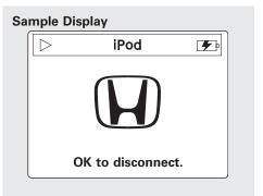
When the iPod is connected and the iPod mode is selected on the audio display, the USB and iPod indicators are shown in the display. After loading, you will see Honda mark\* on the iPod. That means you can only operate your iPod using the vehicle's audio unit.
