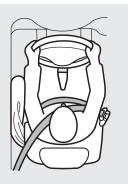
If you ever have a moderate to severe side impact, sensors will detect rapid acceleration and signal the control unit to instantly inflate either the driver's or the passenger's side airbag.
