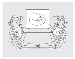
Your vehicle also has cargo hooks on side panel in the cargo area. They are designed to hold light items. Heavy objects may damage the hook. Make sure any items put on each hook weigh less than 2.2 lbs (1 kg).
