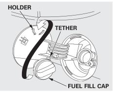
3. Remove the fuel fill cap slowly. You may hear a hissing sound as pressure inside the tank escapes. Place the fuel fill cap in the holder on the fuel fill door. To prevent the fuel fill cap from becoming lost, it is attached to the fuel filler with a tether.
