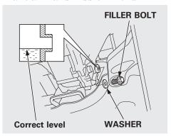
Check the fluid level with the transmission at normal operating temperature and the vehicle on level ground.
