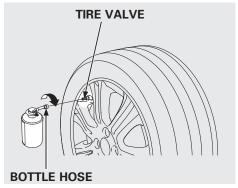
5. Screw the sealant filler hose onto the tire valve. Make sure the bottle remains upright to ensure all of the sealant flows into the tire.
