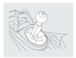
The manual transmission is synchronized in all forward gears for smooth operation. It has a lockout so you cannot shift directly from fifth to reverse. When shifting up or down, make sure you push the clutch pedal down all the way, shift to the next gear, and let the pedal up gradually. When you are not shifting, do not rest your foot on the clutch pedal. This can cause the clutch to wear out faster.
