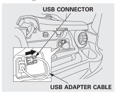
1. Open the upper glove box, and pull out the USB adapter cable.
