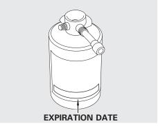
4. Remove the sealant bottle and check the expiration date on the label. If the date has expired, do not continue. Have your vehicle towed to the nearest Honda service center. In Canada or the continental U.S.A. simply call 1-800-465-PLUS (7587) for Honda Plus Roadside Assistance.
