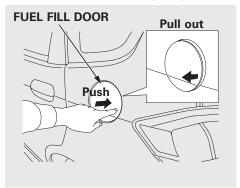
2. Outside of the vehicle, push on the right side edge of the fuel fill door in the middle. The fuel fill door will pop up slightly. Pull it outward to open it.
