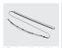
Place the top of the wiper blade on the end of the blade assembly, and slide the blade onto the assembly.
