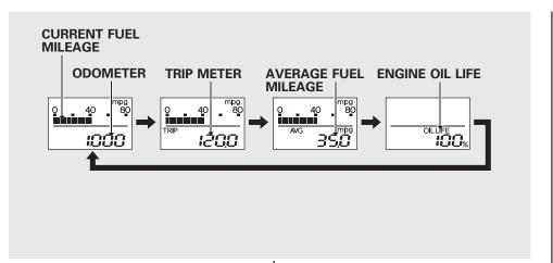
The information display consists of two segments. The upper segment displays current fuel mileage, maintenance item code(s), and the lower segment displays the trip meter, odometer, average fuel mileage, and engine oil life. To switch the display, press and release the select/reset knob repeatedly. When you turn the ignition switch to the ON (II) position the last selection is displayed.
