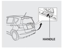
To open the tailgate, pull the handle, then lift up.
