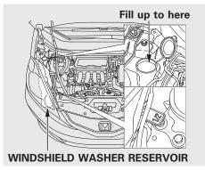
On U.S. models: To check the windshield washer fluid level, open the hood and look the windshield washer reservoir located behind the right headlight. You will see a " 1/2" mark on the reservoir.
