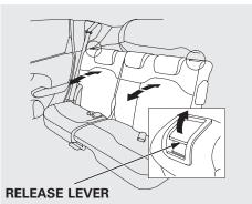
You can adjust the angle of the rear seat-backs separately. To change the seat-back angle, pull up the release lever on the outer side of the seat-back.
