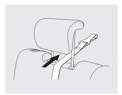
5. Lift the head restraint (see page 94), then route the tether strap through the legs of the head restraint and over the seat-back, making sure the strap is not twisted.
