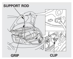
3. Holding the grip, pull the support rod out of its clip. Insert the end into the designated hole in the hood.
