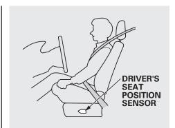
The driver's advanced front airbag system includes a seat position sensor under the seat. If the seat is too far forward, the airbag will inflate with less force, regardless of the severity of the impact.
