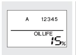
3. Press the select/reset knob for about 10 seconds. The engine oil life and the maintenance item code(s) will blink.
