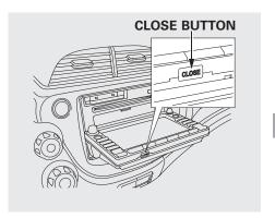
To return the screen to the upright position, press the CLOSE button on the edge of the screen panel. Do not use the folded screen as a tray. If you put a cup, for example, on the screen, the liquid inside the cup may spill on the screen when you go over a bump.
