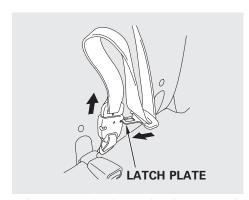
When you fold down the driver's side rear seat, use the latch plate to release the center seat belt from the detachable anchor (see page 99). Allow the seat belt to retract into the holder on the ceiling, and store the buckles in it.
