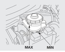
The fluid level should be between the MIN and MAX marks on the side of the reservoir. If the level is at or below the MIN mark, your brake system needs attention. Have the brake system inspected for leaks or worn brake pads/shoes.
