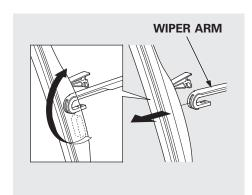
• Pivot the blade assembly toward the wiper arm until it releases from the wiper arm.
