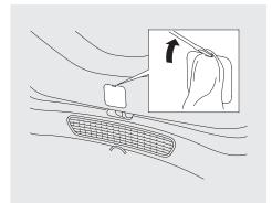
On Sport model and Canadian LX model If the power door lock system cannot unlock the tailgate, unlock it manually.
