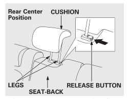
When a passenger is seated in the rear center seating position, the center head restraint should be adjusted up or down, to match the passenger's height.
