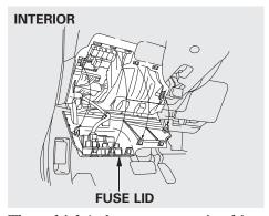
The vehicle's fuses are contained in two fuse boxes.
