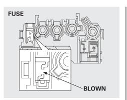
3. Check each of the large fuses in the under-hood fuse box and the interior fuse box by looking through the top at the wire inside.
