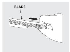
3. Remove the blade from its holder by grabbing the tabbed end of the blade. Pull firmly until the tabs come out of the holder. 4. Examine the new wiper blades. If they have no plastic or metal reinforcement along the back edge, remove the metal reinforcement strips from the old wiper blade, and install them in the slots along the edge of the new blade.
