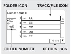
You can also select a track/file directly from a track list on the audio display. Press the AUDIO button to show the audio display, then touch the Track List icon. The track list menu appears on the display.
