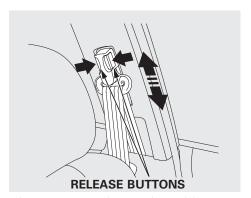
The front seats have adjustable seat belt anchors. To adjust the height of an anchor, squeeze the two release buttons, and slide the anchor up or down as needed (it has four positions). Never place the shoulder portion of a lap/shoulder belt under your arm or behind your back. This could cause very serious injuries in a crash.
