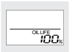
4. Press the select/reset knob for another 5 seconds. The maintenance item code(s) will disappear, and the engine oil life will reset to "100."
