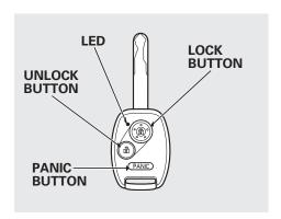
On Sport model and Canadian LX model LOCK — Press this button once to lock all doors and the tailgate. Some exterior lights will flash once. When you push LOCK twice within 5 seconds, the horn will sound to verify that the doors and the tailgate are locked and the security system (if equipped) has set. You cannot lock the doors and the tailgate if any door or the tailgate is not fully closed or the key is in the ignition switch.
