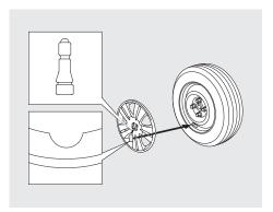
2. Align the valve mark on the wheel cover to the tire valve on the wheel, then install the wheel cover.
