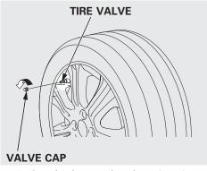
1. Park vehicle on a level surface in a safe place. Set shifter lever into PARK and engage the parking brake. Turn hazard light on. Remove valve cap from tire valve.
