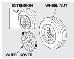
8. On all models except Sport and Canadian LX model with manual transmission, remove the wheel cover by carefully prying under its edge with the flat tip of the extension.
