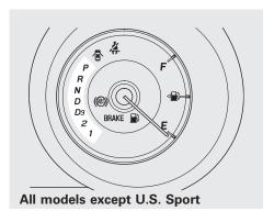
If the malfunction indicator lamp comes on along with the "D" indicator, there is a problem with the automatic transmission control system. Avoid rapid acceleration, and have the transmission checked by your dealer as soon as possible.
