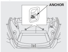
1. After properly securing the child seat (see page 45), lift the head restraint, then route the tether strap over the seat-back and through the head restraint legs.
