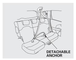
The lap/shoulder belt in the center seating position on the rear seat is equipped with a detachable seat belt that has two parts: a small latch plate and an anchor buckle.
