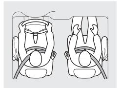
Your vehicle also has side airbags to help protect the upper torso of the driver or a front seat passenger during a moderate to severe side impact (see page 28 for more information on how your side airbags work).
