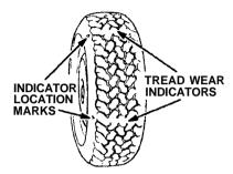
⚠ WARNING Driving on worn-out tires is very hazardous, and will reduce braking effectiveness, steering accuracy and traction.
