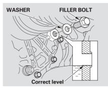
Check the fluid level with the transmission at normal operating temperature and the vehicle sitting on level ground. Remove the transmission filler bolt and carefully feel inside the bolt hole with your finger. The fluid level should be up to the edge of the bolt hole. If it is not, add Honda Manual Transmission Fluid (MTF) until it starts to run out of the hole
