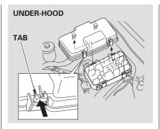
The under-hood fuse box is located in the engine compartment on the driver's side. To open it, push the tabs as shown.
