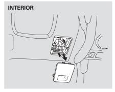
The interior fuse box is underneath the steering column. To remove the fuse box lid, pull it toward you and take the lid out of its hinges.
