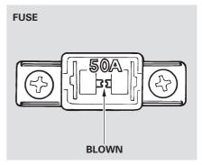
3. Check each of the large fuses in the under-hood fuse box by looking through the top at the wire inside. Removing these fuses requires a Phillips-head screwdriver.
