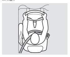
Your car is equipped with side airbags for the driver and a front seat passenger. The airbags are stored in the outer edges of the front seat-backs, and both are marked "SIDE AIRBAG."
