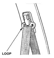
Dirt build-up in the loops of the seat belt anchors can cause the belts to retract slowly. Wipe the insides of the loops with a clean cloth dampened in mild soap and warm water or isopropyl alcohol.
