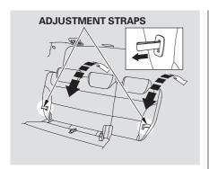
The left and right halves of the third seat-back can be adjusted separately. To adjust the angle, pull the adjustment strap on the outside of each seat-back, move the seat-back to the desired position, and release the adjustment strap. Let the seat-back latch in the new position.
