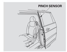
On EX, EX-L and Touring models Each sliding door has a pinch sensor on the front edge. Do not damage this sensor, or the power sliding door may not operate properly.
