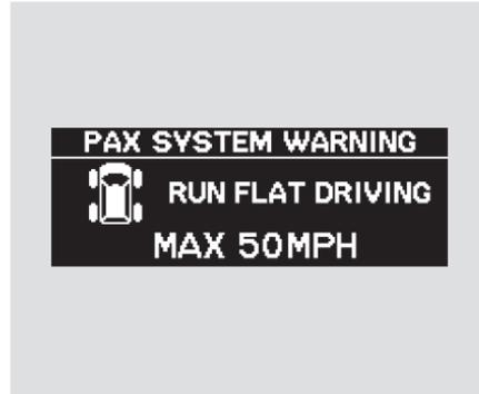
The above message shows that you are driving your vehicle on a flat tire, and should observe the “RUN FLAT DRIVING” speed limit of 50 mph (80 km/h). Drive to your nearest Honda dealer or authorized Michelin PAX system dealer, or call the PAX help hotline at 1-877-PAXTIRE (1-877-729-8473).
