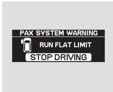
If you see the above message on the multi-information display, you have reached the limit of run flat driving, and you should stop driving immediately. Be aware that if you continue to drive, the noise and vibration level from the tire will increase significantly, and the tire may no longer be repairable.
