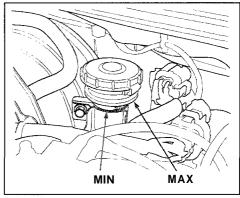
The fluid should be between the MIN and MAX marks on the side of the reservoir. If it is not, add brake fluid to bring it up to that level. Use the same DOT3 or DOT4 brake fluid from a sealed container specified for the brake system.
