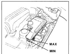
The fluid should be between the MIN and MAX marks on the side of the reservoir. If it is at or below the MIN mark, it indicates a possible problem in the ABS. Have the dealer inspect the system and add fluid.
