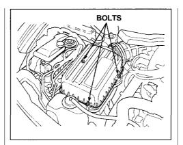
The air cleaner element is inside the box on the passenger's side of the engine compartment. To replace it:
