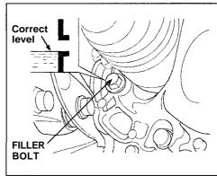
Check the oil level a couple of minutes after shutting off the engine. Make sure the car is on level ground. Remove the transmission filler bolt. The oil level should be up to the edge of the bolt hole. Feel inside the bolt hole with your finger. If you do not feel any oil, slowly add oil until it starts to run out of the hole. Reinstall the filler bolt and tighten it securely.
