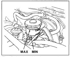
The fluid should be between the MIN and MAX marks on the side of the reservoir. If the level is at or below the MIN mark, it is an indication that your brake system needs attention. Have the brake system inspected for leaks or worn brake pads.
