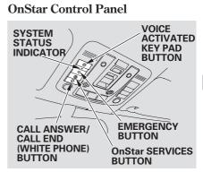
The OnStar buttons and indicator are located on the ceiling near the front ceiling light. (Oň)
