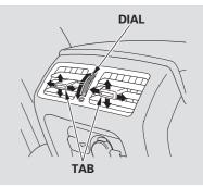
You can adjust the direction of the air coming from the rear vents in the back of the center console by moving the tab in the center of each vent up-and-down and side-to-side.
