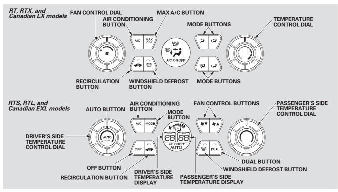
On RTS, RTL, and Canadian EXL models, see pages 128 and 129 for information on automatic climate control and semi-automatic operation.
