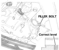
Check the oil level a couple of minutes after shutting off the engine. Make sure the car is on level ground. Remove the transmission filler bolt. The oil level should be up to the edge of the bolt hole. Feel inside the bolt hole with your finger. If you do not feel any oil, slowly add oil until it starts to run out of the hole. Reinstall the filler bolt and tighten it securely.
