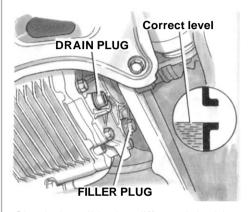
Check the oil in the differential with the car sitting level. Remove the oil filler plug and check that the oil level is up to the edge of the hole.
