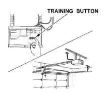
3. Press the Training button on the garage door opener unit until the light next to the button comes on, then release it. The light may blink, or come on and stay on. You then have approximately 30 seconds to complete the following steps.
