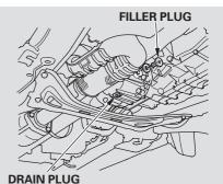
Check the fluid in the transfer assembly with the vehicle sitting on level ground. Remove the filler plug and check that the fluid level is up to the edge of the filler plug hole. If it is not, slowly add proper fluid until it starts to run out of the hole. Reinstall the filler plug and tighten it securely. Tightening torque: 33 lbf·ft (45 N·m , 4.6 kgf·m)
