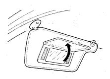
The light next to the mirror will come on when the headlight switch is in either ON position.
