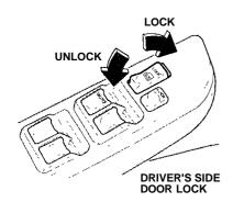
Press the front of the lock button to lock all the doors, and the rear of the button to unlock all doors. The lock knob on each door controls only that door. Push the lock knob down to lock, and pull it up to unlock. To lock any passenger's door from the outside, push the lock knob down and close the door.
