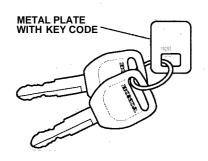
The key code number is stamped on the metal plate attached to the key ring.
