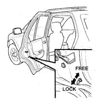
This is done by depressing the lever shown in the illustration. To disengage the lock, open the door from the outside and raise the lever.
