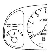
If the light flashes, it means the computer controlling the transmission has found a problem. Have the automatic transmission
