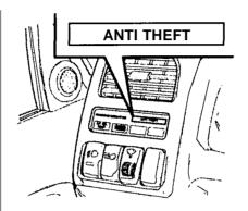
The system sets automatically when the passenger doors, tailgate door, and hood are locked. The ANTI-THEFT light comes on for ten seconds to indicate the system is set.
