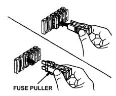
4. Check the smaller fuses in the under-hood fuse box and all the fuses in the interior fuse boxes by pulling out each fuse with the fuse puller provided in the under-hood fuse box
