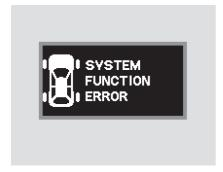
If you see this message, the tire pressure monitor shows a "SYSTEM FUNCTION ERROR" message. The system may not be able to detect or signal low tire pressure as intended. Also, the tire pressure readings will not be displayed. Have your vehicle checked by a dealer as soon as possible.
