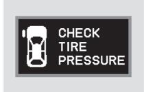
When any of the tires have low pressure, the low tire pressure indicator on the instrument panel comes on, and the multi-information display also interrupts the current display and shows a "CHECK TIRE PRESSURE" message. You can see one or more of the low pressure tire positions highlighted in the display along with this message.
