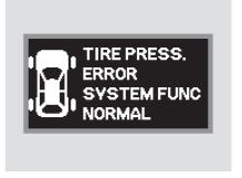
When any of the tires have low pressure, the tire pressure monitor shows a "TIRE PRESS. ERROR SYSTEM FUNC NORMAL" message.
