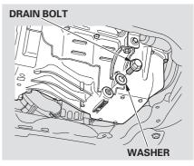
4. Remove the oil drain bolt and washer from the bottom of the engine. Drain the oil into an appropriate container.
