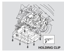
3. Remove the nine holding clips with a flat-tipped screwdriver, then pull the cover down.
