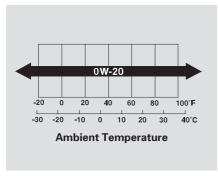
A very low-viscosity, fuel-efficient 0W-20 oil is the preferred engine lubricant for your Civic Hybrid. This special oil is formulated to help your engine use less fuel. It is available at vour Honda dealer. A 5W-20 oil may be used if 0W-20 is not available.
