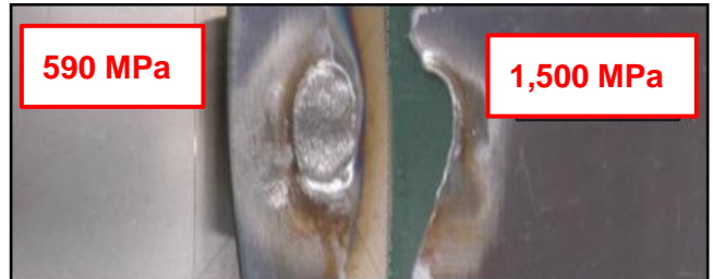
Tensile Test Results of MAG Welded 1,500 MPa Steel
