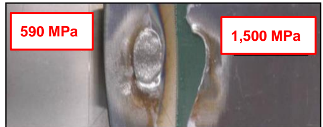
Tensile Test Results of MAG-Welded 1,500 MPa Steel
