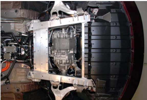
Removing the underbody covers that protect components from dirt and damage reveals the drive motor, located between the front wheels.
