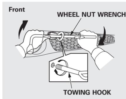
2. Remove the towing hook and wheel nut wrench placed behind a cover under the cargo area.
