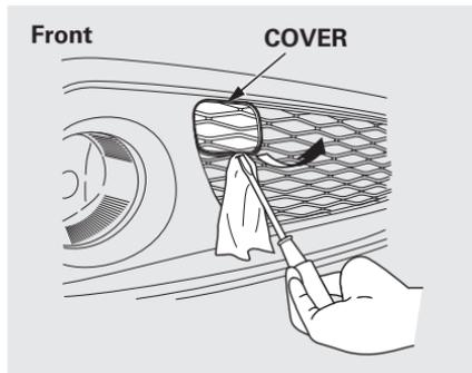
1. Remove the cover, put cloth on the edge of the cover to prevent scratches and carefully pry with a small flat-tip screwdriver or a metal fingernail file.
