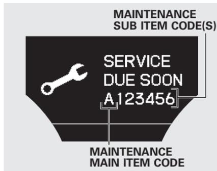
When the remaining engine oil life is 15 to 6 percent, the multi-information display shows a “SERVICE DUE SOON” message along with the maintenance item code(s) indicating the main and sub items required at the time of the oil change. Refer to page 542 for a complete list of the maintenance main items and sub items.
