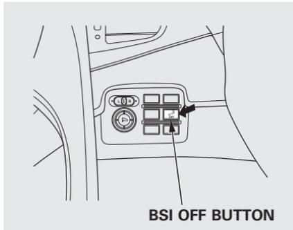
To turn the system off, press the BSI OFF button when the power mode is set to ON with the engine start/stop button. The BSI indicator on the instrument panel glows amber, indicating that the system is turned off. The multi-information display indicates that the system is off.
