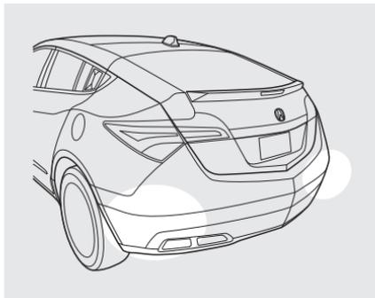
Radar sensors, located underneath each corner of the rear bumper, detect objects. Do not cover this area with labels or stickers of any kind. Always keep this area is free of any kind of dirt every time you get in the vehicle.
