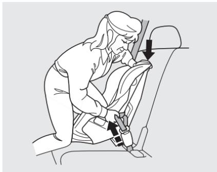
4. After confirming that the belt is locked, grab the shoulder part of the belt near the buckle, and pull up to remove any slack from the lap part of the belt. Remember, if the lap part of the belt is not tight, the child seat will not be secure.
