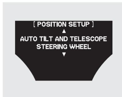
When “AUTO TILT AND TELESCOPE STEERING WHEEL” is set to “ON,” the steering wheel automatically moves fully up when you turn the ignition switch to the LOCK (0) position and remove the key (or the vehicle is in VEHICLE OFF mode on models with keyless access system).
