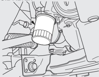
3. Remove the oil filter, and let the remaining oil drain. A special wrench (available from your dealer) is required.
