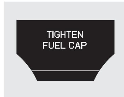
Your vehicle's on board diagnostic system will detect a loose or missing fuel fill cap as an evaporative system leak. The first time a leak is detected a “TIGHTEN FUEL CAP” message appears on the multi-information display. Turn the engine off, and confirm the fuel fill cap is installed. If it is, loosen it, then retighten it until it clicks at least once.
