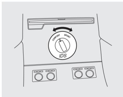
Turn the Integrated Dynamics System (IDS) switch located on the center console to select the comfort and sport mode.
