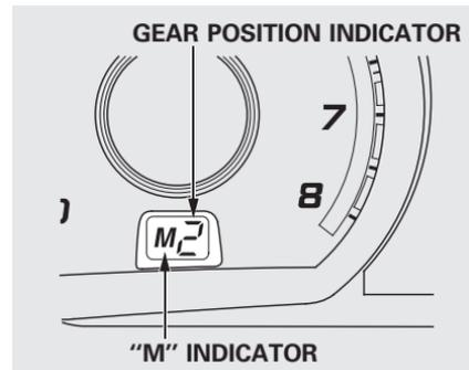
When you move the shift lever from "D" to "S" and pull either paddle shifter, the gear position indicator displays "M" along with the selected gear number.
