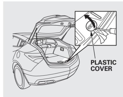
5. The spare tire is stored underneath the rear cargo area. Remove the plastic cover on the cargo area lining to access the shaft for the spare tire hoist.
