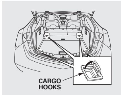
To secure cargo, use the four floor hooks in the cargo area. Make sure all stored items are secured before driving.
