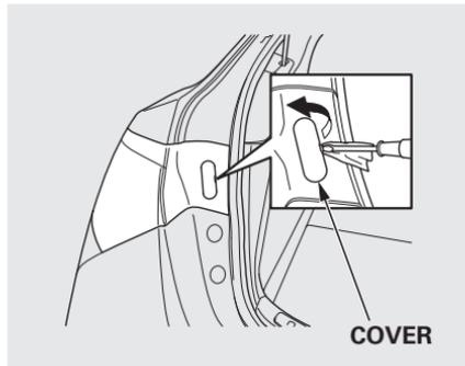
1. Open the tailgate. Use a flat-tip screwdriver protected with a cloth to prevent scratches and pry open the cover.
