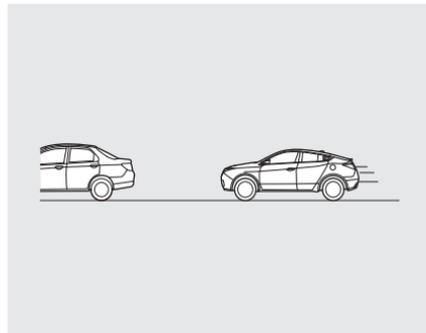
If the system senses a likely collision with a vehicle or object ahead of you, it alerts you with an audible and a visual alarm.
