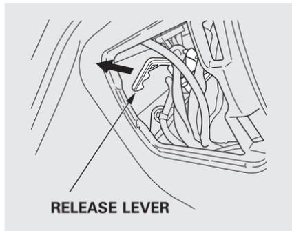
To open the fuel fill door, pull the release lever rearward.
