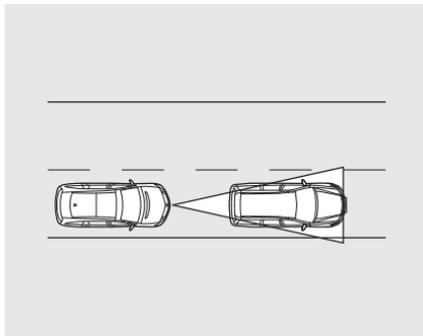
*When a vehicle ahead is within ACC range and going at a steady speed*
