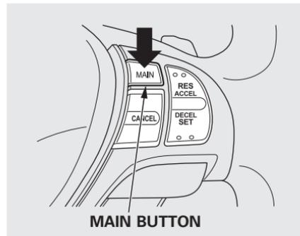
1. Push the MAIN button on the steering wheel. The ACC indicator on the instrument panel comes on, and "ACC" is shown on the multi-information display.
