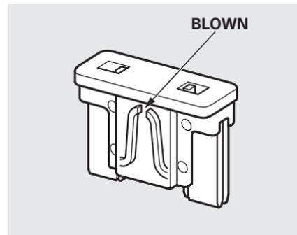
5. Look for a burned wire inside the fuse. If it is burned out, replace it with one of the spare fuses of the same rating or lower.
