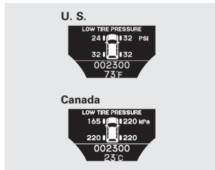
If any of the tires has low pressure, the tire pressure monitor also shows the above message and each tire pressure to warn you about the low tire pressure when you select the display by pressing the INFO button several times.
