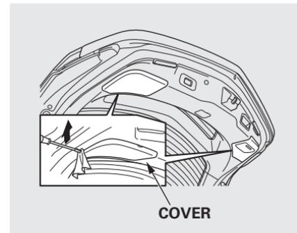
1. Open the tailgate. Place a cloth on the edge of the light assembly cover to prevent scratches. Remove the cover by carefully prying in the notch on its middle edge with a flat-tip screwdriver.
