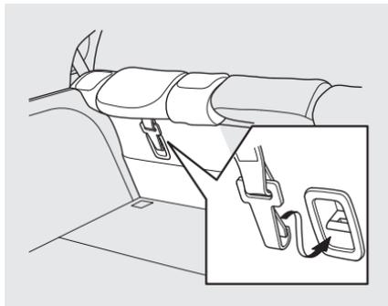
7. Attach the tether strap hook to the tether anchor, then tighten the strap as instructed by the child seat maker.
