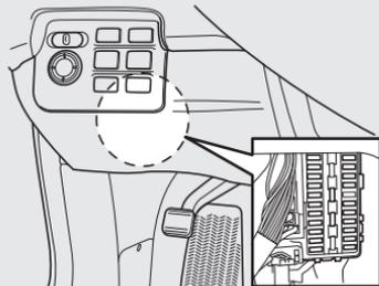
The vehicle's fuses are located in four fuse boxes.
