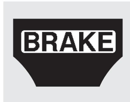
The audible alarm is a constant beeping sound; the visual alert is an amber colored BRAKE message that flashes on the multi-information display. If these alarms come on, take the appropriate means to prevent a collision (apply the brakes, change lanes, etc.).
