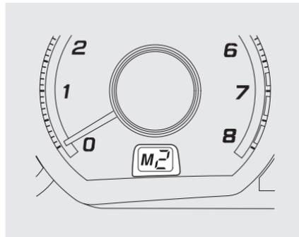
Using a paddle shift mode, the gear position indicator shows you the selected gear number (see page 482).
