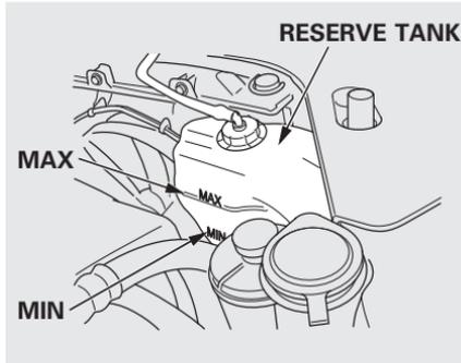
Look at the coolant level in the radiator reserve tank. Make sure it is between the MAX and MIN lines. If it is below the MIN line, see **Adding Engine Coolant** on page [548](#) for information on adding the proper coolant.
