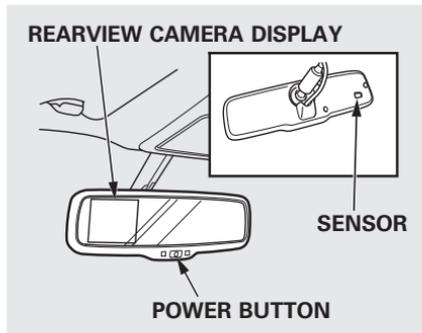
You can turn the camera display on and off by pressing the power button when the shift lever is in reverse. The camera display turns on every time you shift to reverse, even if you turned it off the last time.
