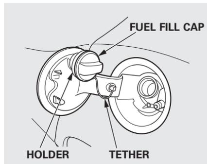
4. Remove the fuel fill cap slowly. You may hear a hissing sound as pressure inside the tank equalizes. Place the cap in the holder on the fuel fill door.
