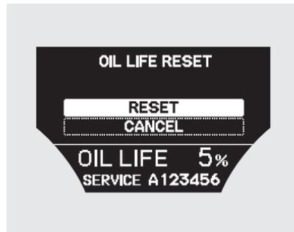
4. Select “RESET” by pressing the INFO (▲/▼) button, then press the SEL/RESET button to reset the engine oil life display. The maintenance item code(s) will disappear, and the engine oil life will reset to “100.” If you want to cancel the oil life reset mode, select “CANCEL.”
