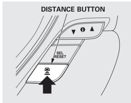
To switch from ACC to cruise control, press the distance button on the steering wheel, and hold it for 1 second.
