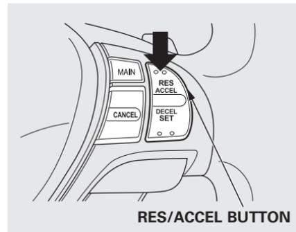
The set speed can be increased by using the RES/ACCEL button or the accelerator pedal.
