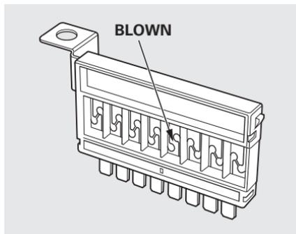
Also check the combined fuse box in the under-hood fuse box.
