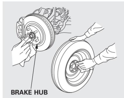
13. Before mounting the spare tire, wipe any dirt off the mounting surface of the wheel and hub with a clean cloth. Wipe the hub carefully; it may be hot from driving.
