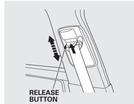
The front seats have adjustable seat belt anchors. To adjust the height of an anchor, press and hold the release button and slide the anchor up or down as needed (it has four positions).
