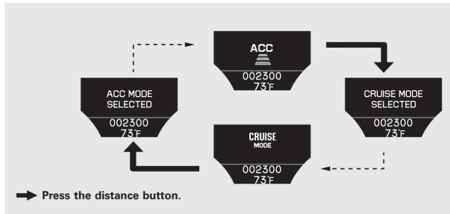
When you press the button, you will see CRUISE MODE SELECTED on the multi-information display for 2 seconds. To switch back to ACC, press and hold the distance button again for 1 second.
