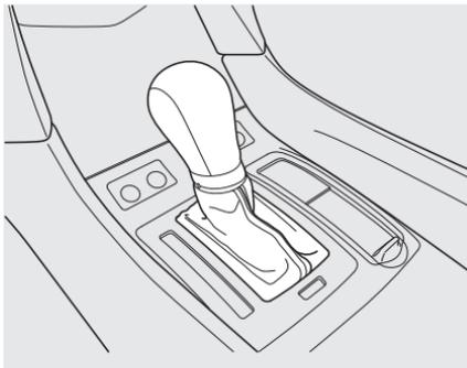
To shift from Park to any position, press firmly on the brake pedal, and press the release button on the front of the shift lever, then move the lever. You cannot shift out of Park when the ignition switch is in the LOCK (0) or ACCESSORY (I) position.
