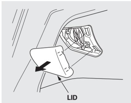
If there is a problem with the power door lock system and you cannot unlock the driver's door, use the release lever behind the left side cover in the cargo area.
