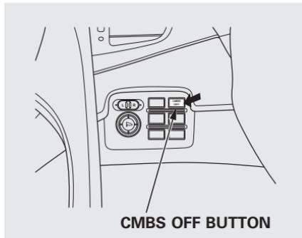
To turn the CMBS off, press the CMBS OFF button under the driver's side vent for about 1 second. When you do this, a beeper sounds, a CMBS indicator on the instrument panel comes on, and a CMBS OFF message appears on the multi-information display. To turn the system back on, press the button again for about 1 second.
