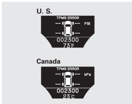
If there is a problem with the TPMS, the tire pressure monitor shows a “TPMS ERROR” message and the tire pressure readings are not displayed. If this happens, you will first see a system warning message “CHECK TPMS SYSTEM” on the multi-information display.
