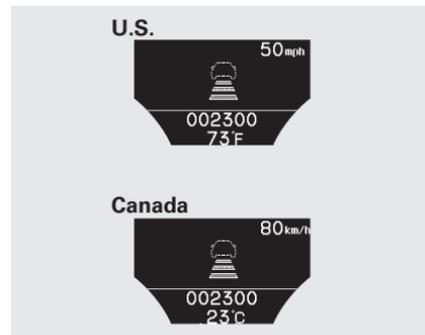
When that vehicle changes lanes or goes out of ACC range, a beeper sounds once. If there is no vehicle ahead of you within ACC range, a dotted-line vehicle icon will be on the multi-information display. To set the ACC beeper on or off, see page [103](#).
