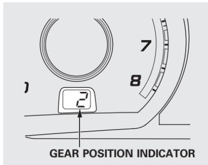
Each time you pull + (right), the transmission shifts to a higher gear. Pull - (left) to downshift. You will see the selected gear number on the instrument panel.
