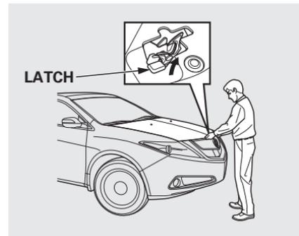
2. Put your fingers under the front edge of the hood near the center. Slide your hand to your left until you feel the hood latch handle. Push this handle up until it releases the hood. Lift up the hood.
