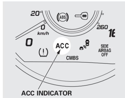
The ACC indicator (orange) normally comes on for a few seconds when you select the ON mode by operating the engine start/stop button (see page 194). If it comes on at any other time, there is a problem in the ACC system. If this happens, take the vehicle to your dealer to have it checked.
