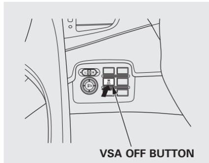
This button is under the driver's side vent. To turn the VSA system on and off, press and hold it until you hear a beep.
