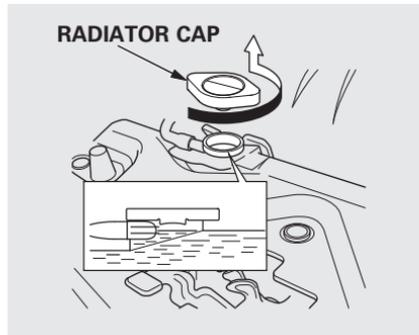
3. Remove the radiator cap by pushing down and turning counterclockwise.
