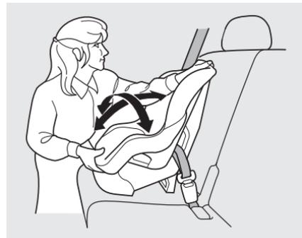
5. Push and pull the child seat forward and from side-to-side to verify that it is secure enough to stay upright during normal driving maneuvers. If the child seat is not secure, unlatch the belt, allow it to retract fully, then repeat these steps.
