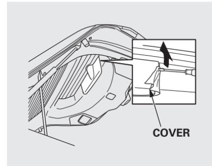
1. Open the tailgate. Place a cloth on the edge of the light assembly cover to prevent scratches. Remove the cover by carefully prying in the notch on its edge with a flat-tip screwdriver.
