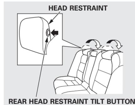
3. Push the rear head restraint tilt buttons on the head restraints to pivot the head restraints down.
