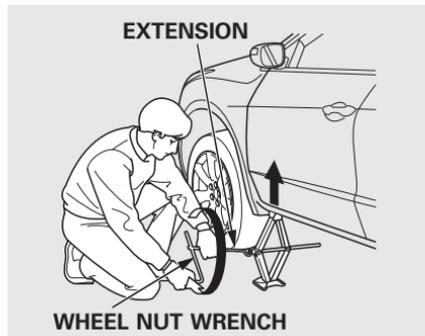
11. Use the extension and the wheel nut wrench as shown to raise the vehicle until the flat tire is off the ground.
