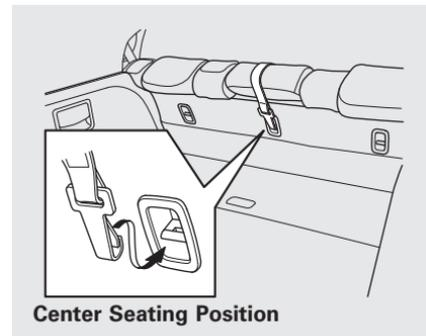
1. For the center seat, lower the head restraint, then route the tether strap over the head restraint and seat-back.
