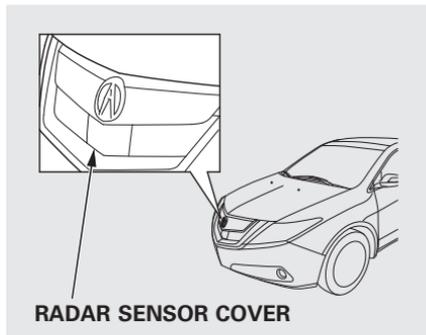
The radar sensor cover is located under the Acura emblem in the front grille. If the radar sensor cover is covered with mud, dirt, dead leaves, wet snow, etc., or if you put a sticker on it, the CMBS will automatically shut off, and the CMBS indicator on the instrument panel will come on. You will also see a “CHECK CMBS RADAR SENSOR” message on the multi-information display for about 5 seconds.
