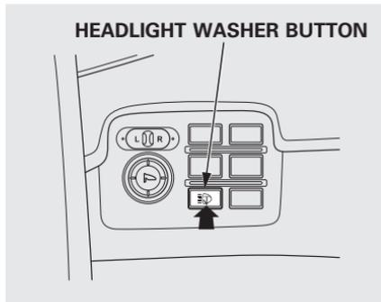
The headlight washers can be operated at any time by pressing the headlight washer button located next to the steering wheel column. The headlights must be turned on to use this button. In addition, the headlight washer operates without pressing the button the first time you turn on the windshield washers with the ignition switch in the ON (II) position.
