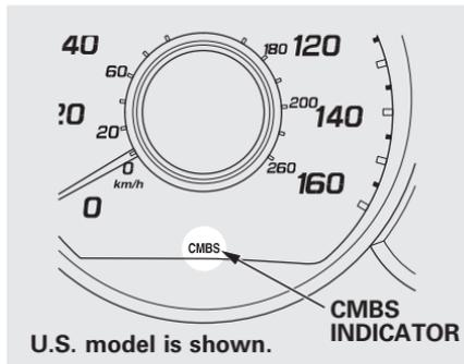
This indicator comes on for several seconds when you select the ON mode by operating the engine start/stop button (see page 194). It also comes on and stays on when you turn the CMBS off by pressing the CMBS OFF button.
