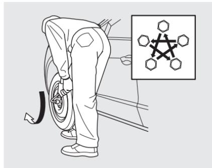
16. Tighten the wheel nuts securely in the same crisscross pattern. Have the wheel nut torque checked at the nearest automotive service facility.
