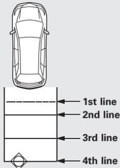
The camera display has parking guide lines that indicate distance from your vehicle.
