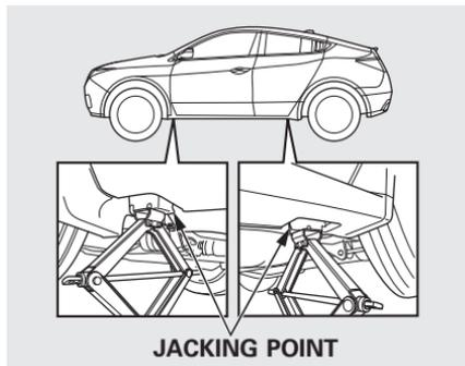
10. Place the jack under the jacking point nearest the tire you need to change. Turn the end bracket clockwise until the top of the jack contacts the jacking point. Make sure the jacking point tab is resting in the jack notch.
