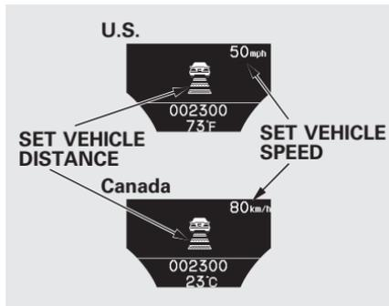
When the speed is set, it is shown along with a vehicle icon and distance bars on the multi-information display. Refer to page [390](#) for how to set and change the set distance between your vehicle and the vehicle ahead of you.
