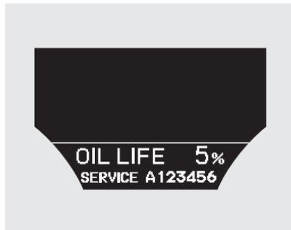
Press the SEL/RESET button on the steering wheel repeatedly to select the engine oil life. The message "SERVICE," along with "5%," and the maintenance item code are displayed on the multi-information display when the calculated engine oil life is 1 to 5 percent (see page [534](#)).
