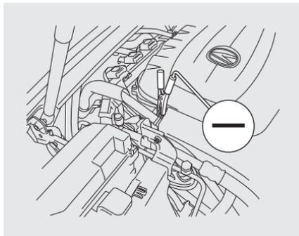
4. Connect the second jumper cable to the negative (-) terminal on the booster battery. Connect the other end to the engine hanger as shown. Do not connect this jumper cable to any other part of the engine.
