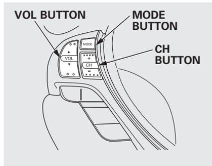
Three controls for the audio system are mounted in the steering wheel hub. These let you control basic functions without removing your hand from the wheel.
