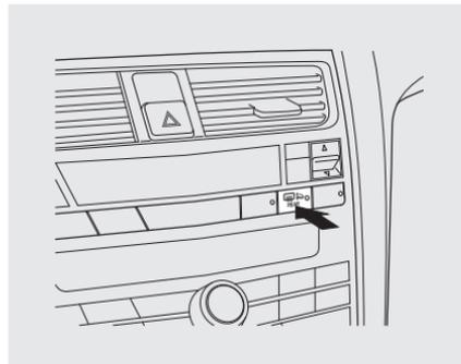
The rear window defogger will clear fog, frost, and thin ice from the window. Push the defogger button to turn it on and off.
