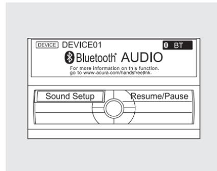
Press the AUDIO button to display the audio control display. Turn the dial to switch the setting between the resume/pause mode and the sound setup mode. Select Sound Setup, then press ENTER to set your selection.
