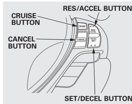
1. Push in the CRUISE MAIN button (models with adaptive cruise control) on the steering wheel. The CRUISE MAIN indicator on green ACC indicator (models with ACC) on the instrument panel comes on.
