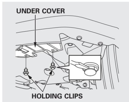
1. Remove the two holding clips with a flat-tip screwdriver.
