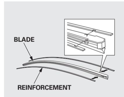
Make sure the two rubber tabs inside the blade fit to each notch of the reinforcement, as shown.
