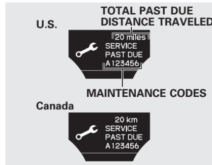
If the indicated required service is not done and the remaining engine oil life becomes 0%, the multi-information display will show a "SERVICE PAST DUE" message, the total distance traveled after the remaining oil life became 0%, and the maintenance item code(s).
