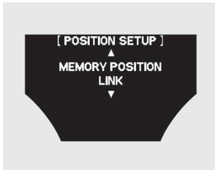
If “MEMORY POSITION LINK” is set to “ON,” the driver's seat, the steering wheel, and outside mirror positions move to the position stored in the memory when you open the driver's door, using the remote transmitter.
