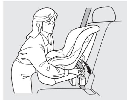
1. With the child seat in the desired seating position, route the belt through the child seat according to the seat maker's instructions, then insert the latch plate into the buckle and remove any slack from the lap portion of the belt.
