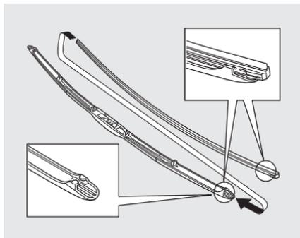
5. Place the top of the wiper blade on the end of the blade assembly, and slide the blade onto the assembly in the direction pointed to by the arrow.
