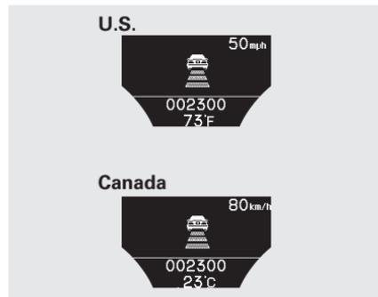
When the system detects a vehicle ahead of you, a beeper sounds once and a solid-line vehicle icon appears on the multi-information display.
