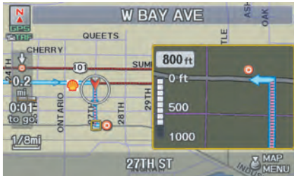
Blue-pink unverified route line (unverified routing on)
