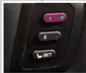
**Note:** Each group of settings is activated by the corresponding remote transmitter (1 or 2) when it's used to unlock the driver's door. When activated, each item begins to adjust before you enter the vehicle.
