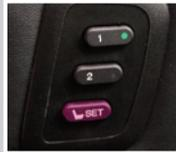
4. **Press and hold** the memory button corresponding to the remote (1 or 2) you are using until you hear two beeps.
