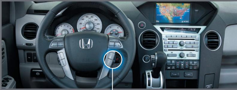
While on the Trip Computer display, press the SEL/RESET button to access trip information. Press either Info (▲/▼) button to toggle through the various screens, or the SEL/RESET button for sub-displays.
