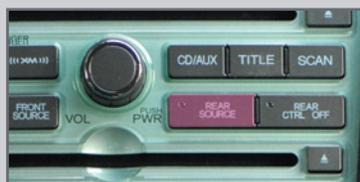
2. **Press** the REAR CTRL OFF button to disable the rear audio controls.
