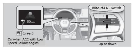
When driving at about 25 mph (40 km/h) or above: Take your foot off the pedal and press the RES/+/SET/– switch up or down when you reach the desired speed. The moment you release the switch, the set speed is fixed, and ACC with Low Speed Follow begins.
