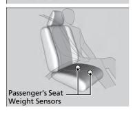
The front passenger's advanced airbag system has weight sensors. The sensors are used for occupant classification to activate or deactivate the front passenger's airbag.
