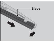
**3.** Slide the blade out of the wiper.
