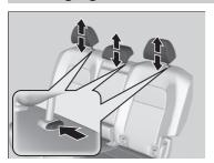
A passenger sitting in the rear seat should adjust the height of their head restraint to an appropriate position before the vehicle begins moving.
