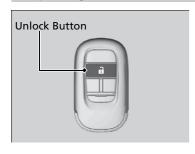
**To open:** Press the unlock button, and then within 10 seconds, press it again and keep it pressed. If the windows stop midway, repeat the procedure.
