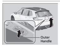
When all the doors are unlocked or you press the tailgate unlock button\* on the remote transmitter, the tailgate is unlocked. Press the outer handle and lift open the tailgate.
