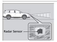
The radar sensor is behind the Honda emblem on the front grille.
