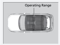
The power system may also start if the keyless remote is close to the door or window, even if it is outside the vehicle.
