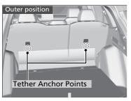
A tether anchor point is provided behind the rear outer seating positions and in the ceiling for the rear center.
