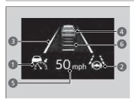
You can see the current state of Adaptive Cruise Control (ACC) with Low Speed Follow, Lane Keeping Assist System (LKAS) and Traffic Jam Assist.
