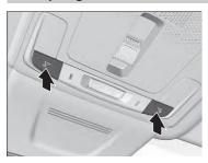
The map lights can be turned on and off by pressing the switches.
