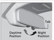
Flip the tab to switch the position.
