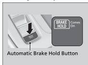
Fasten your seat belt properly, then turn the power system on. Press the automatic brake hold button.
