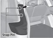
**2.** Pull the taillight carefully until the snap pins are removed from the body grommets.
