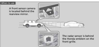
The system starts monitoring the roadway ahead when your vehicle speed is about 3 mph (5 km/h) or above and will search for a vehicle, pedestrian, or moving bicycle in front of you.
