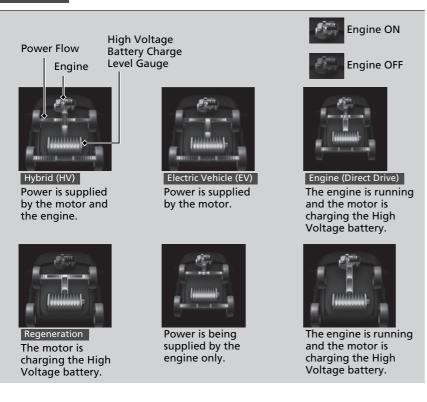
▶ Power Flow/Engine Status Display/High Voltage Battery Charge Level Gauge
