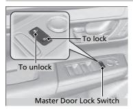
Press the master door lock switch in as shown to lock or unlock all doors, tailgate, and fuel fill door.
