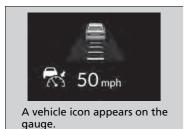
When a vehicle whose speed is slower than your set speed comes in or cuts in front of you and is detected by the radar and the camera, your vehicle starts to slow down.
