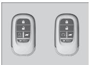
Use the keys to turn on and off the power system, and to lock and unlock the doors, tailgate, and fuel fill door.
